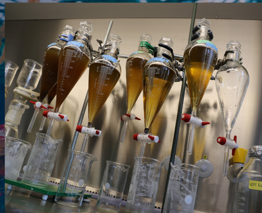
Image 4: Separating funnels to perform a density separation of microplastics from sediments. Photo © K.Beck/IOW.
